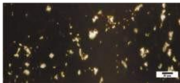
Figure 3. Optical microscopy image of microchannel system coated with Fe 3 O 4 -GSH-PEG-Tf matrix (2.0 mg).
